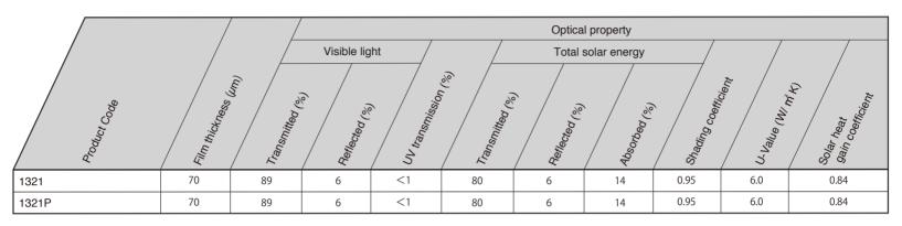
Solar spectrum Ultraviolet rays: 300nm-380nm, Visible light: 380nm-780nm, Total solar energy: 300nm-2500nm The indicated value is measured using 3mm float glass with eachtype of film applied, based on JIS A 5759 The values reported in the data are actual measured values and not guaranteed.
